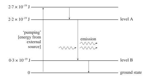
(a) The useful output of the laser results from the transition between level A and level B.
